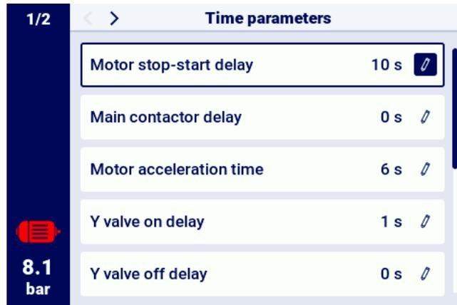
Figure 26: Menu view with time parameter settings for the Inverter configuration
