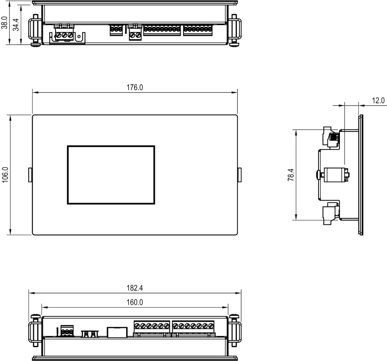
Figure 50: Controller housing drawing
