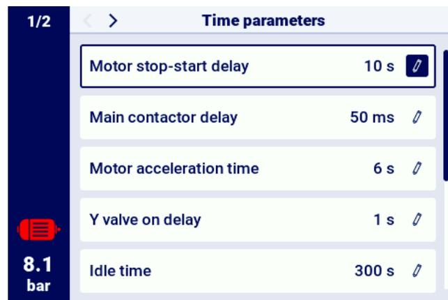
Figure 24: View of the menu with time parameter settings for the Star-Delta configuration
