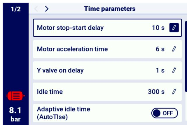
Figure 29: View of the menu with time parameter settings for Direct Start configuration
