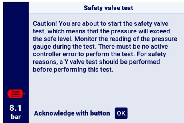
Figure 31: Safety valve test start warning
