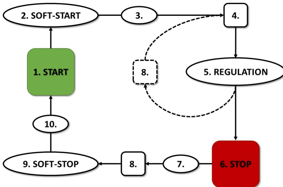
Figure 25: Motor control algorithm
