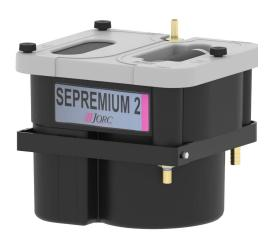
As soon as the condensate enters the SEPREMIUM 2 Serviceable, it is filtered through the various filter elements. The oil absorbing elements combine different types of adsorption technologies, assuring a result of less than 5 ppm residual oil content at the exit can be achieved.
